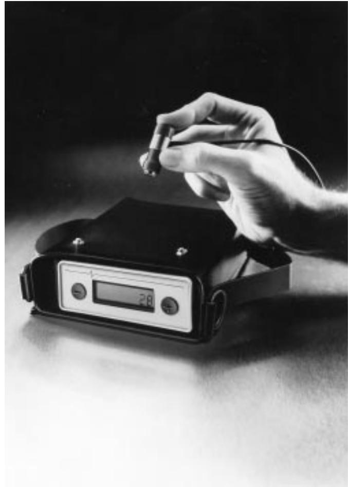
**FIG. 1 Ultrasonic Thickness Gage**
